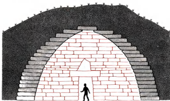
Sometimes a chamber was hollowed under a hill, and stones used to strengthen walls and roof.
